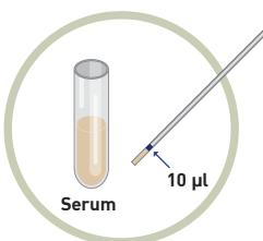
**2** Apply 10 µl of the sample into the sample hole.
